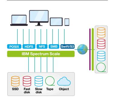
IBM Spectrum Scale provides a single scale-out environment for the entire data center.
